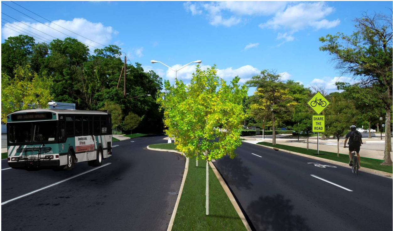
Example 3: Modifications include adding sidewalks with buffers, “Share the Road” signs, “sharrow” markings, and landscaping the median.
