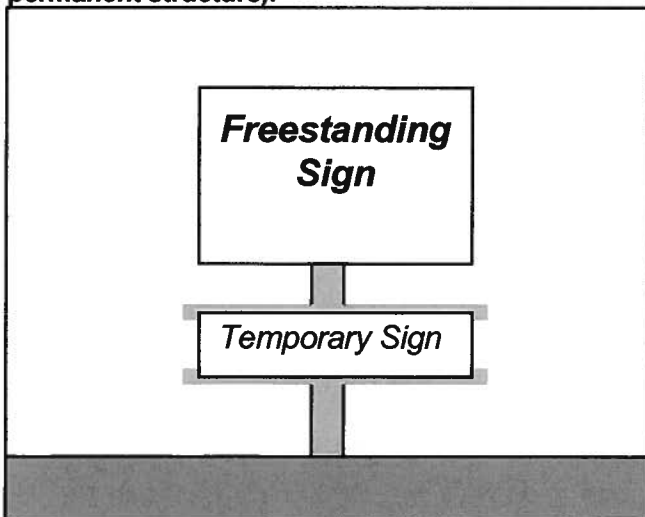
Figure 3. Permitted- Additional supports (which do not touch the ground) are used to affix a temporary sign at all corners to a freestanding sign (single permanent structure).
